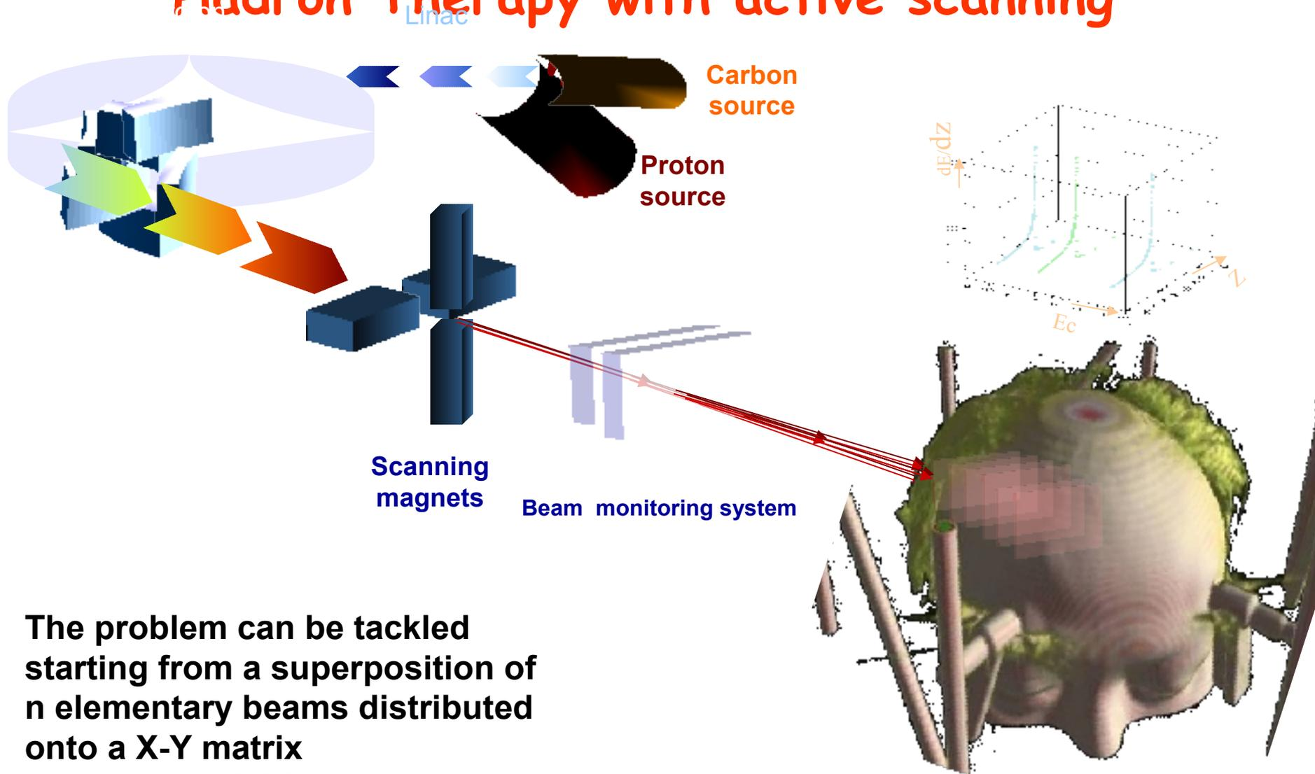
The problem can be tackled starting from a superposition of  $n$  elementary beams distributed onto a X-Y matrix + angular variables
