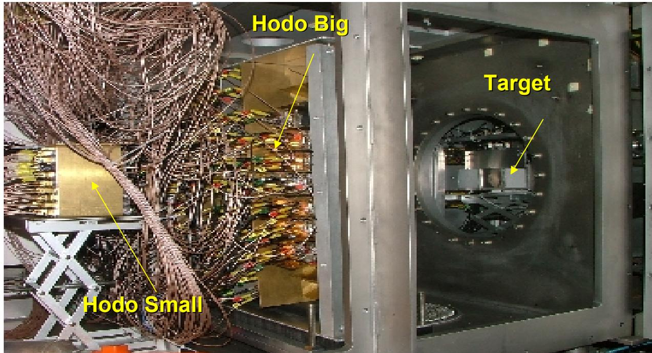
***Hodo-big***: 89 three-fold telescopes  $50\ \mu\text{m} + 300\ \mu\text{m}$  Silicon detectors  $3 \times 3\ \text{cm}^2$  surface followed by a 6 cm long CsI(Tl)  $\theta_{lab}$  between  $\pm 4.5^\circ$  and  $\pm 16.5^\circ$ .
